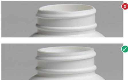
If the closure seal does not work properly, it compromises the integrity of the contents, negates the protection of the child resistant closure, and the product may be in recall danger. Product waste, lost production time, and replacement of product will eat into profits.
