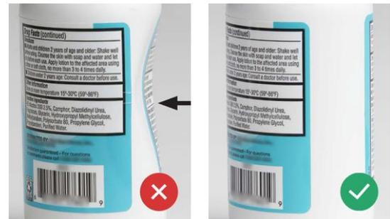
This causes bottle deformities and problems on filling lines and after filling. We determine how much plastic is necessary to protect and contain the products. We also recommend the correct sealing liner, avoiding potential issues and save money.
