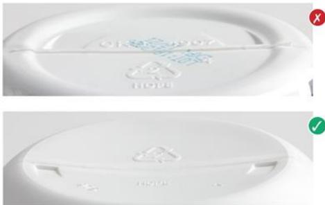
When excess flash material remains on the bottom of the bottle, it results in instability and causes the bottle not to stand straight on the shelf. This also result in a poor printing surface and a mediocre brand impression.
