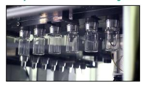
ISBM is used to manufacture bottles that have small to medium bodies and relatively small necks. We use ISBM to manufacture all of our Polyethylene Terephthalate (PET) bottles.
