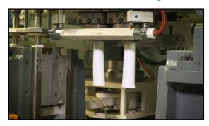
The EBM process is used to manufacture large-size, High Density Polyethylene (HDPE), Low Density Polyethylene (LDPE), and Polypropylene (PP) bottles with large necks.
