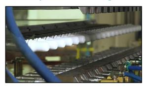
IBM is ideal for the production of HDPE, LDPE, and PP bottles that have small bodies and relatively small necks. IBM is used when manufacturing bottles with very tight neck tolerances.
