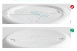
Excess bottom flash may not be removed from the bottom of the bottle and can cause the bottles to be unstable and not stand straight on the shelf. This can result in a poor printing surface and a mediocre brand impression.
