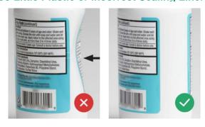
Causes bottle deformities and problems on filling lines, and after it is filled. We can determine how much plastic is necessary to protect and contain your product. We can recommend the correct sealing liner, avoiding potential issues and save money.
